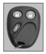
button once will unlock the driver's door. The interior lamps will come on. Pressing unlock again within three seconds will cause the remaining doors to unlock.
